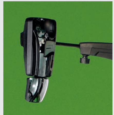
↑ Mirrors with electric adjustment and defrosting.
