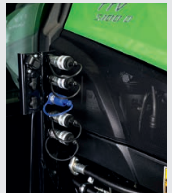
↑ Mid-mounted hydraulics ways for front implements.
