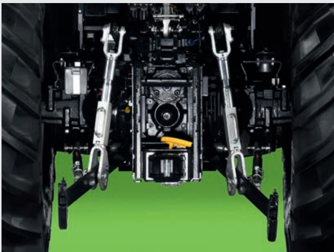
↑ Standard three-point hitch for higher lifting capacity.
