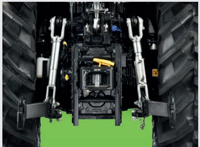
↑ Compact three-point hitch for narrow track.
