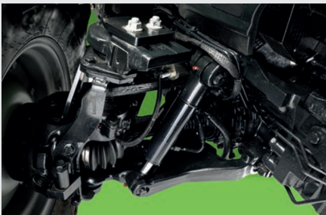
↑ Suspended front axle with front brakes.
